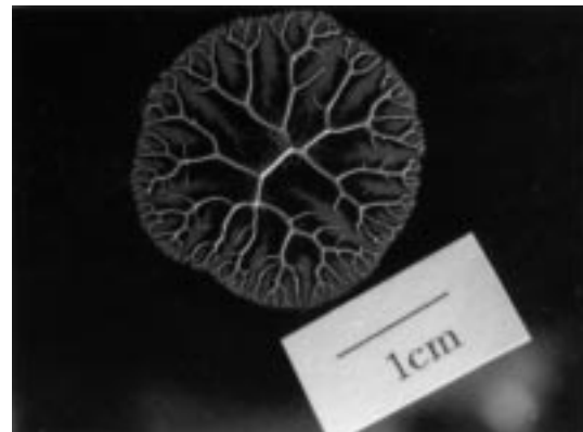
Fig. 1. A pattern formed by air displacing oil paint in the lifting Hele-shaw cell.
